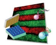
Paint by number? Magnetic nanoparticles (MNPs) coated with distinct biomolecules (see picture) can be assembled onto nanoelectrodes on a template under the control of magnetic and electric fields. The MNP—biomolecule conjugates can then be transferred from the template to a biocompatible polymer substrate. Arbitrary nanopatterns can be fabricated by the magnetic electric lithography process over a large area with a resolution down to 10 nm.
