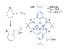
Low-pressure catalyst: A novel dizinc complex (1) having a macrocyclic ancillary ligand shows remarkable activity for the copolymerization of carbon dioxide and cyclohexene oxide, at only one atmosphere of CO<sub>2</sub>. TON = turnover number; TOF = turnover frequency.
