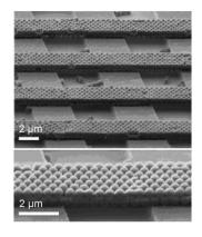
Make a stand: The formation of stable and ordered free-standing particle bridges and hollow capsule structures with controllable sizes and geometries is demonstrated by combining the directed assembly of submicrometer particles, transfer printing, and supramolecular layer-by-layer assembly.
