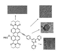
Four from one: Nanoscale ribbons, tubes. vesicles, and platelets can be formed from the self-assembly of a single covalent unit, which is based on an amphiphilic perylene diimide functionalized with a terpyridine ligand (see picture). The assembly diversity arises from the encoding of multiple inputs through hydrophobic interactions and metal coordination.
