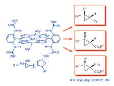
Toss the olefin into the porphyrin: The development of chiral cobalt(II)-porphyrin catalysts by straightforward coupling processes has made possible the additions of diazocarbonyl compounds to a broad spectrum of olefins to access functionalized cylopropanes. The cyclopropanation reactions demonstrate high product yields, exceptional diastereoselectivity, and excellent enantiocontrol.
